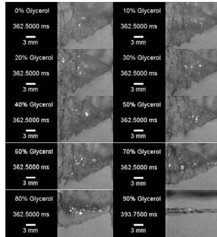
Figure 6. Developed stage of spray for different fluids
